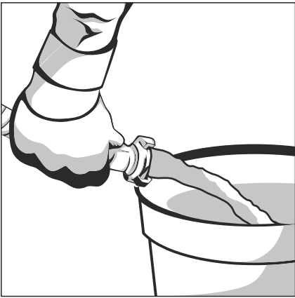
13. Material should flow freely through the hose. If material blocks in the hose it should be diluted.
