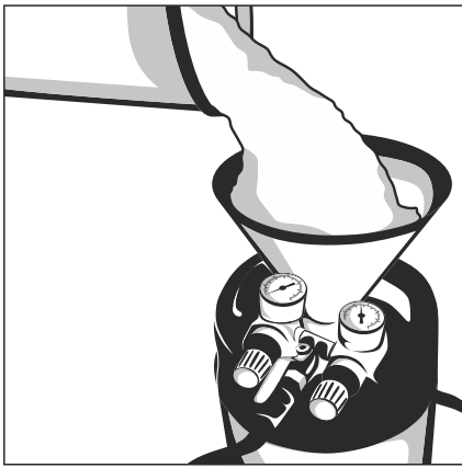
10. Open the tank. Pour material with proper consistency (liquid) to the tank and close it.
