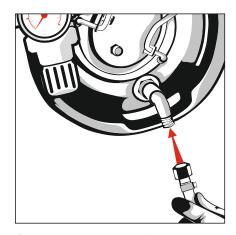
7. Connect the material hose to the tank.
