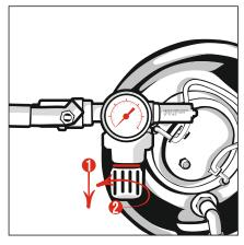
2. Pull the reducer knob with your hand, then turn it counter-clockwise all the way (the reducer knob is often factory unscrewed).
