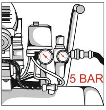
4. Set the pressure on the compressor to 5 BAR.
