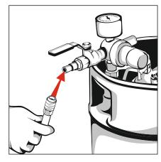
3. Connect the air supply hose to the compressor.
