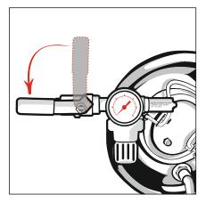
1. Screw the reducer to the tank with a 19 mm wrench and open the ball valve.
