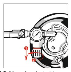
Pull the reducer knob with your hand, then turn it counter-clockwise all the way (the reducer knob is often factory unscrewed).
