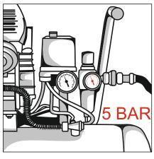
4.Set the pressure on the compressor to 5 BAR. You can also use a small electric compressor.
