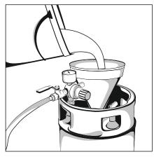
6. Pour the prepared brine solution into the tank.
