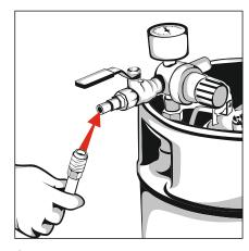
Connect the air supply hose to the compressor. It is recommended to use an oil-free compressor.
