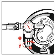
9.Set the tank pressure to a value within the range of 1.5 - 2.5 BAR.
