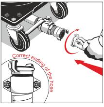
5. Attach to the bottom exhaust hose 25 mm ended with GEKA claw coupling with a strong clamp bracket.
