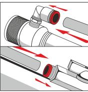
Installation of air hose. Press flange near screwed elbow slipping hose ball valve
