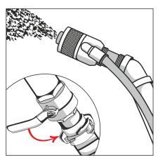
18. Open material ball valve on the lance. You can start working!
