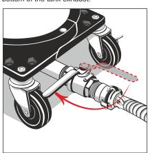
13. Close material valve near bottom exhaust of the tank.
