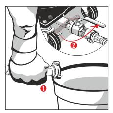
10. Position material hose above a bucket or different container and open ball valve at bottom of the tank exhaust.
