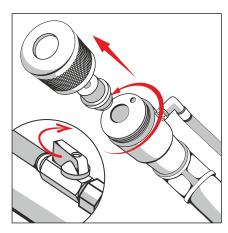
14. Screw small ball valve at the lance then unscrew the nut of nozzle and remove nozzle from the lance.
