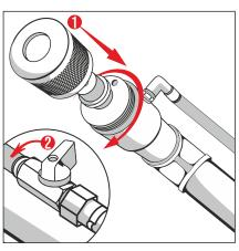
17. Put appropriate nozzle to the lance and screw the nut. Next open small ball valve on the lance.
