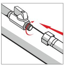
6. Connect air hose to small ball valve at the lance.
