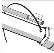
Screw together both parts of the lance Attach the small air valve and hose to
