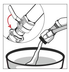
16. Position the lance with removed nozzle above a container. Next, open ball valve of material on the lance until material flows freely. When material flows through the lance close the ball valve of the material on the lance.
