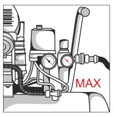
4. Set maximum pressure on the compressor. Compressor should have at least 2 pistons in V mode and capacity 50 L.
