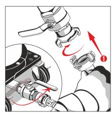
15. Connect material hose to the lance. Next, open ball valve near bottom exhaust of the tank.
