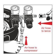
3. Connect air supply hose to compressor and air supply hose to lance.
