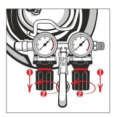
2. Using your hand pull the knob handle of the reductor and turn it left until you will feel resistance. Repeat this action with the second knob handle (manometers are often fabrically unscrewed).
