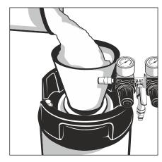
9. Open the tank, pour material to the tank and close it. Material should be diluted as material producer recommends.
